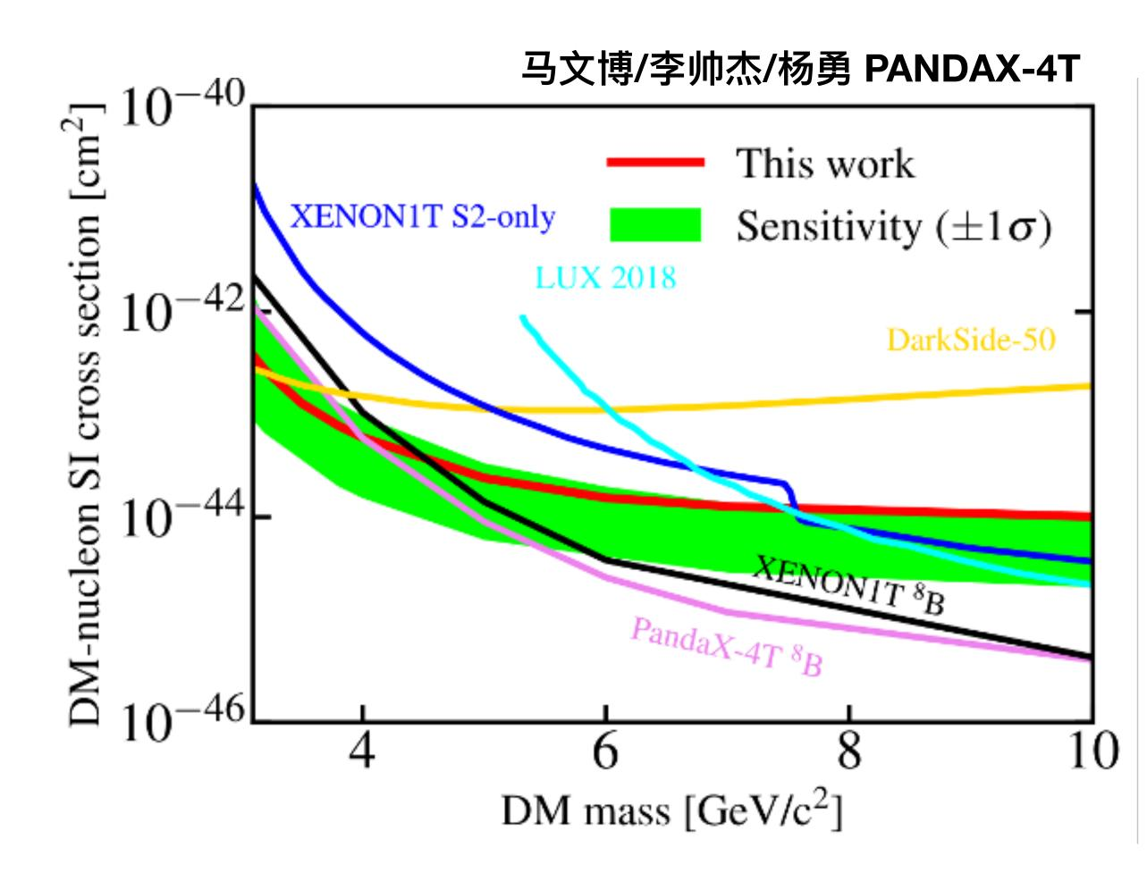
For liquid xenon TPC, use S2-only channel to reduce the energy threshold
