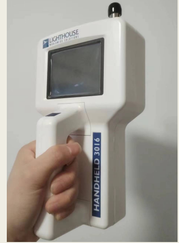
The cleanliness is monitored by Lighthouse Handheld 3016
