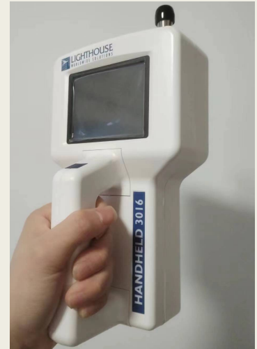
The cleanliness is monitored by Lighthouse Handheld 3016
