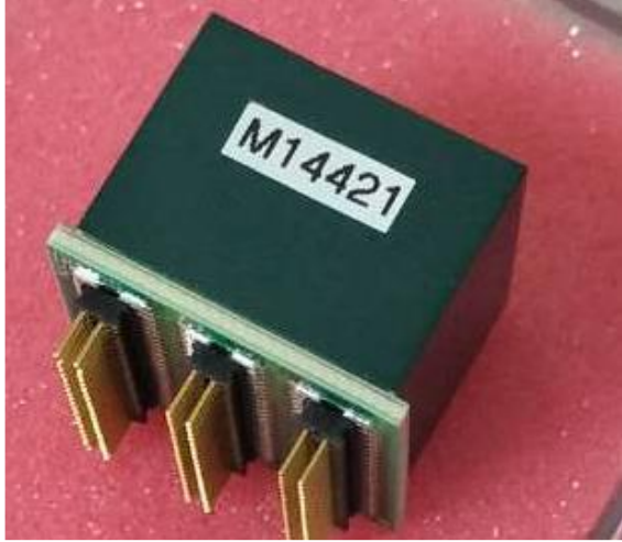
Redlen CZT晶体模块 2 \times 2 \times 1.5 \text{ cm}^3 Pixel pitch = 1.72 mm
