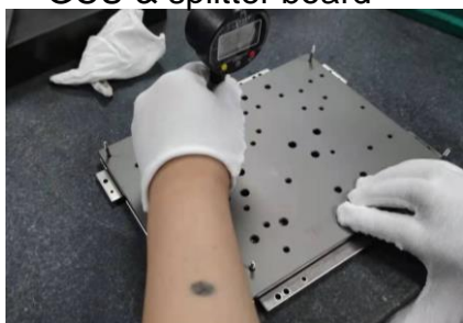
flatness check of the heat sink
