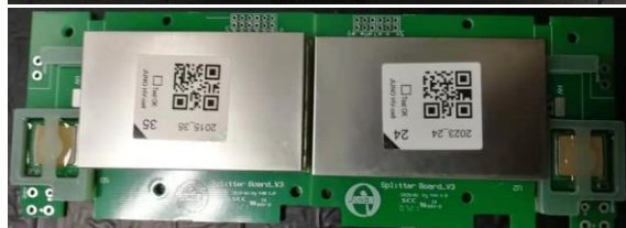
GCU & splitter board
