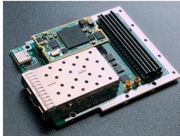
Mini-WR FMC for System-level clock synchronization
