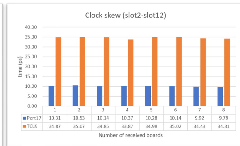
Receiver is fixed at slot 2, add more adjacent AMC boards
