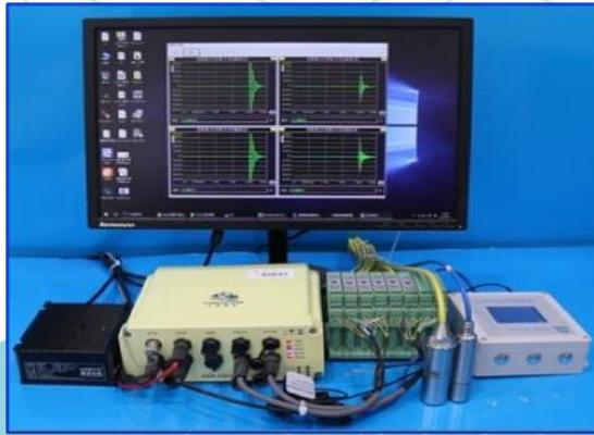
microseismic monitoring system
