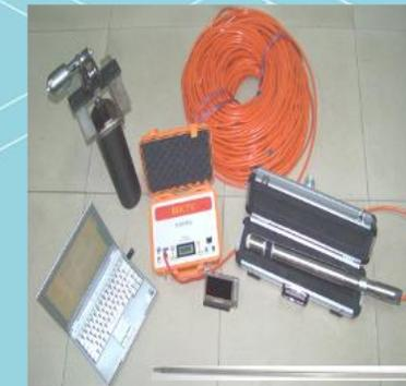
rock cracking monitor
