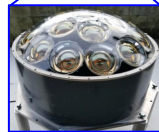
~102 mPMT modules x19, 3" PMTs each
