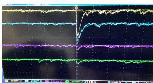
Scintillation coincidence signal of the WLS
