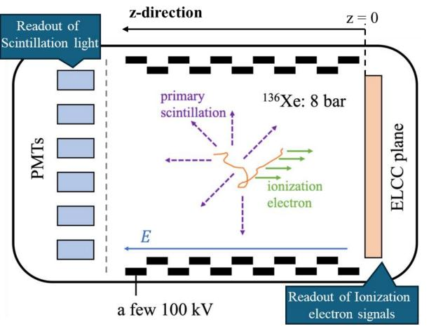
▲ AXEL detector schematic
