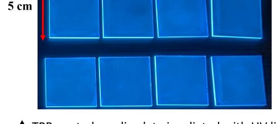
▲ TPB-coated acrylic plate irradiated with UV light
