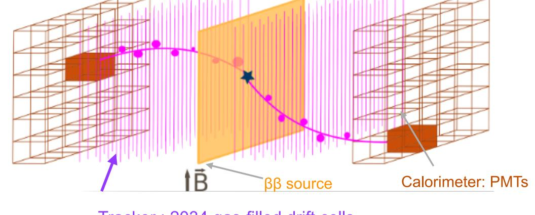
Tracker: 2034 gas-filled drift cells Helium: 95% Inert gas → reduce energy loss Argon:1% Low ionisation energy → avalanche propagation Ethanol: 4% quenching → stop avalanche
