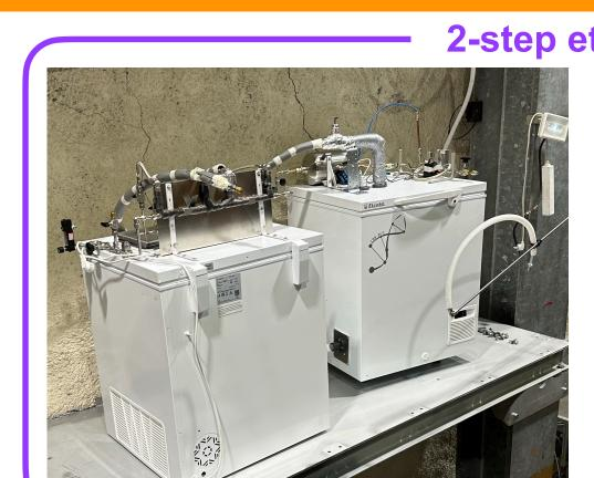
2-step ethanol removal system Condense ethanol from 4% to 70ppm with cryogenic bubbler Remaining 70ppm cleaned by adsorption to < 1ppm
