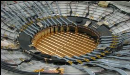
Ring Imaging Cerenkov (RICH) measure Z , E
