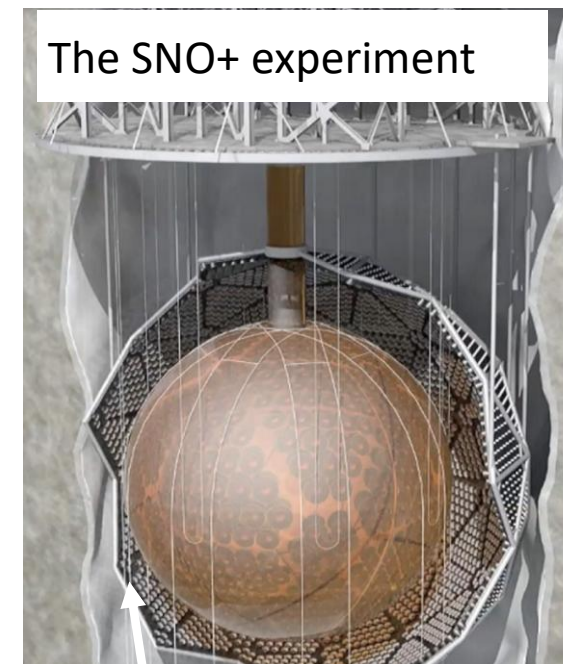
Water shielding (7000 tonnes UPW)
