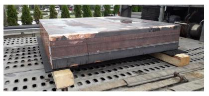
Cu for the cryostat and the most internal shield layer
