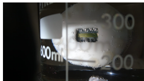
Holmes array chip in KOH solution
