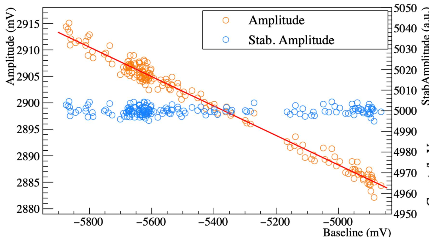
We employ fixed energy pulses to correct for drifts in the thermal gain
