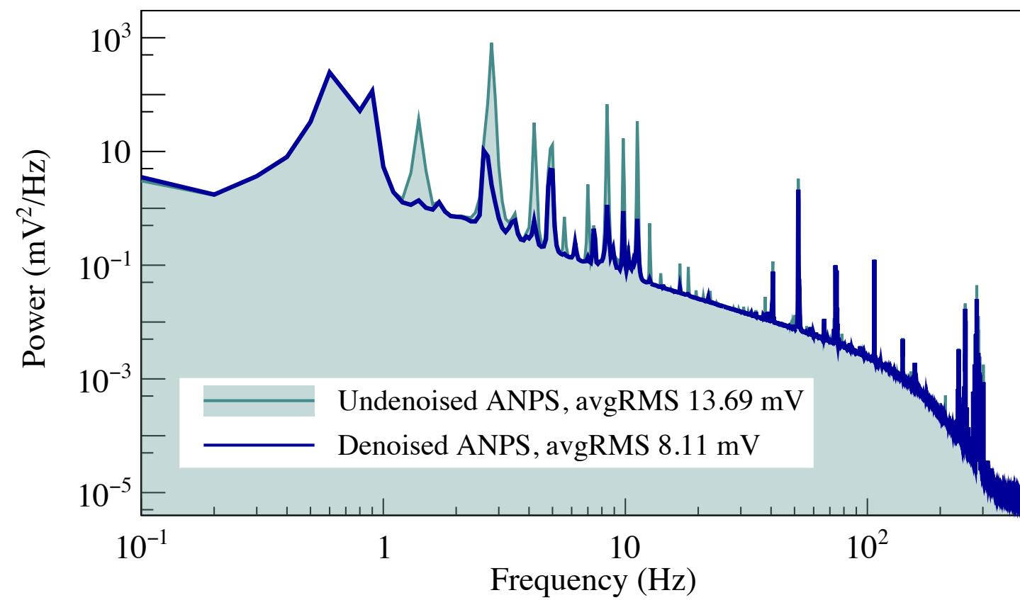
Noise is mitigated correlating vibrations with measurements obtained with auxiliary devices, i.e. microphones, accelerometers, seismometers
