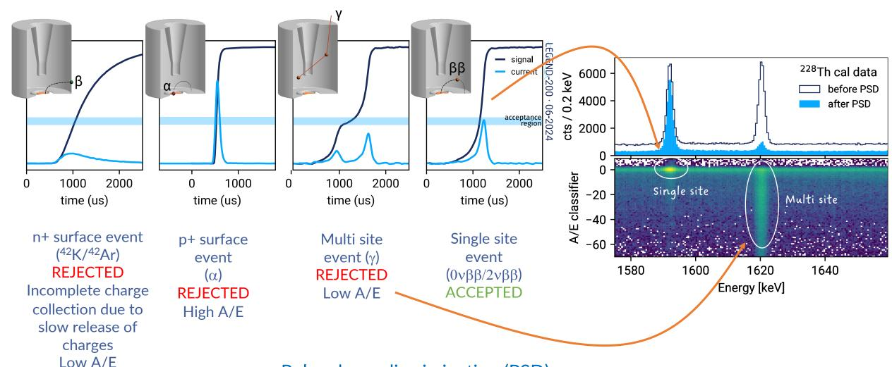
Pulse shape discrimination (PSD): based on the signal risetime and amplitude
