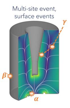
Background rejection: in addition to careful material selection and handling during installation, Liquid Argon instrumentation and Muon Veto + Pulse Shape Discrimination
