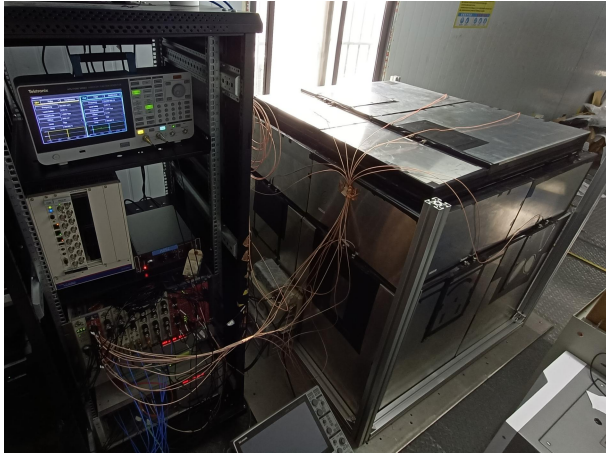
EC-PCGe system Muon detector installed in the container
