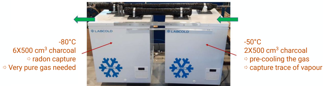
Radon capture system
