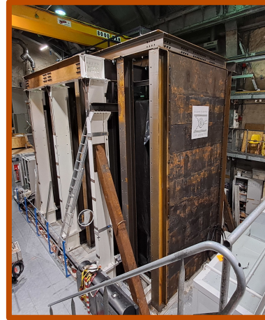
Iron shielding (18 cm) ambient gamma
