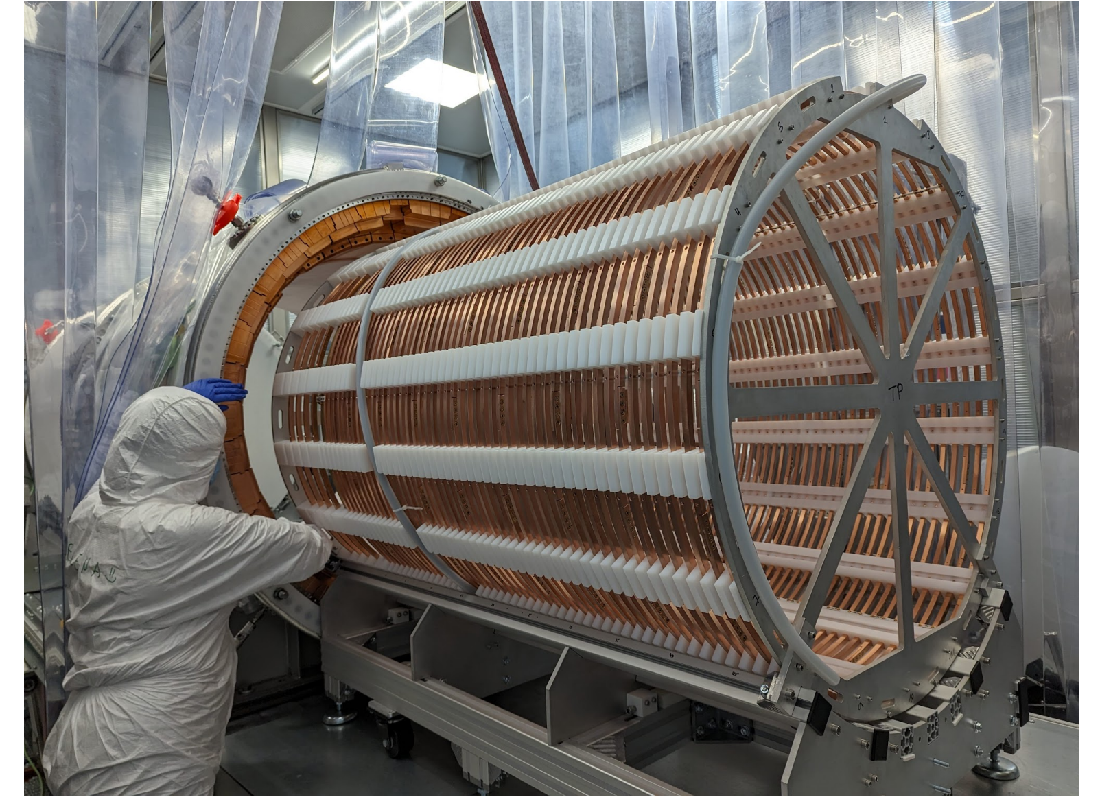
Detector field cage
