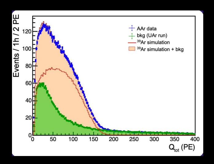
With a prototype, we measured the energy spectra of atmospheric argon and UAr from the DarkSide-50 production batch (1kg argon)
