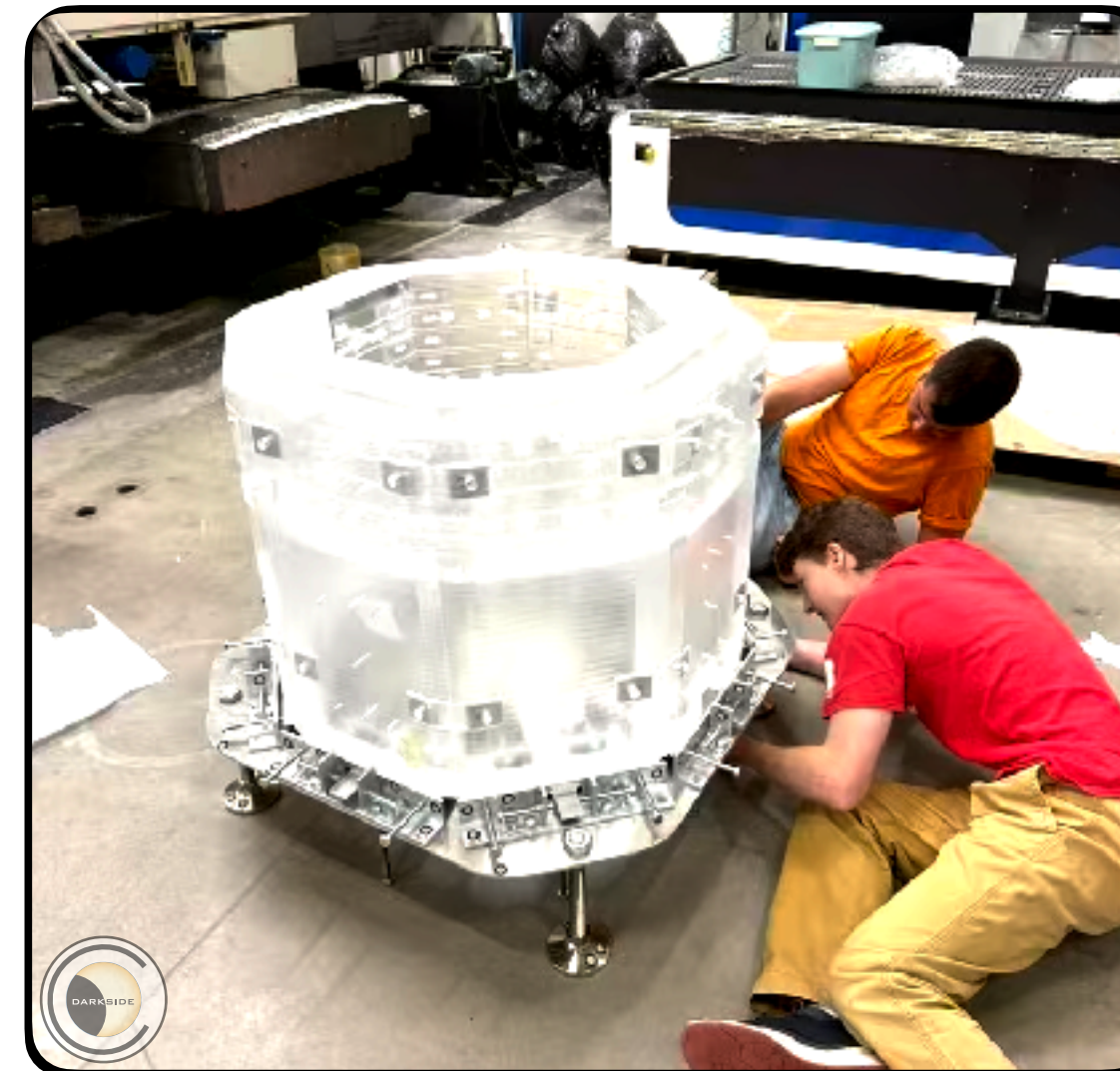
Test Assembly of the DS-Mockup Barrel
