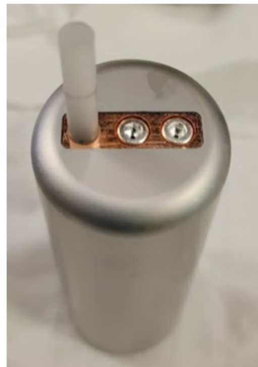
Rod with Cu-Sapphire Axle Inserts
