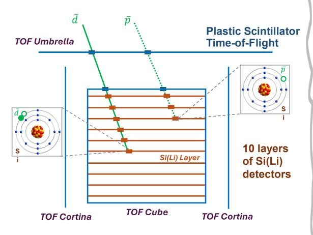
*Time-of-flight* system: measures velocity, incoming angle and dE/dx, fast trigger
