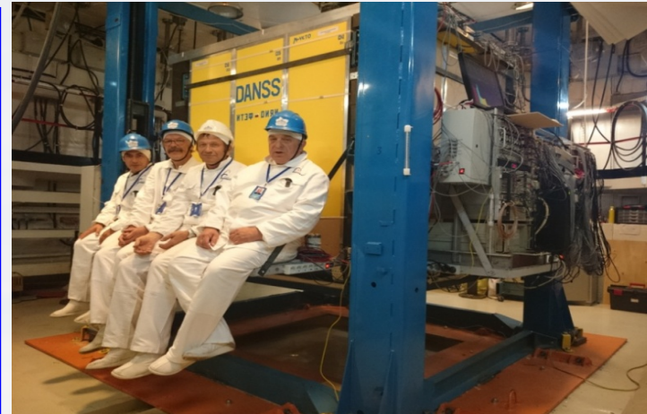
DANSS on a lifting platform Two week cycle of up/down position
