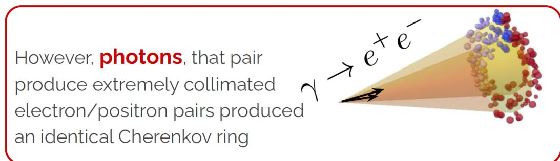
**MiniBooNE Cherenkov detector unable to distinguish photons and electrons, and unable to detect hadronic final-state particles below Cherenkov threshold.**
