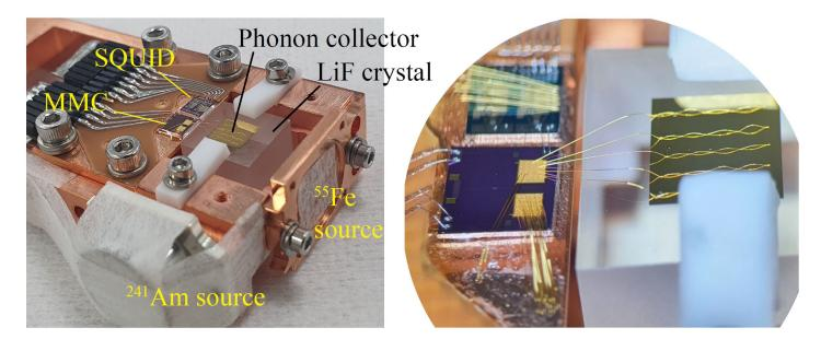
Measurement with internal <sup>55</sup>Fe and <sup>241</sup>Am calibration sources
