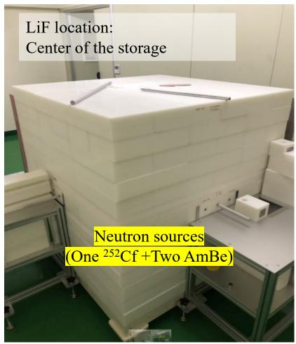
Neutron irradiation at KRISS Week exposure  $\rightarrow \sim 20$  Bq in a LiF
