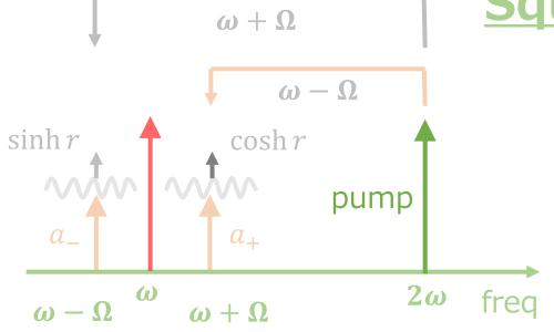
Injecting the carrier and pump beams into a non-linear crystal, either amplitude or phase fluctuation increases and the other one decreases.
