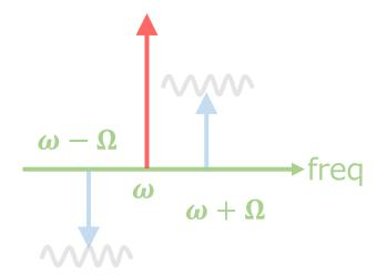
Quantum-noise sidebands are out-of-phase to carrier.
