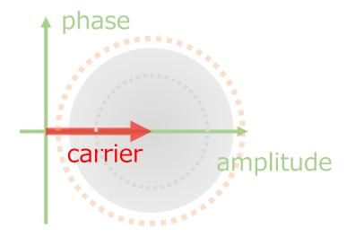
A non-degenerated OPA works as a phase-insensitive amplifier.
