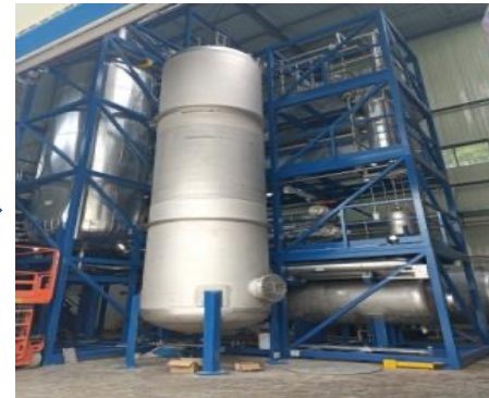
Distillation to remove radioactive impurities
