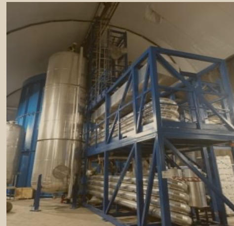
Gas stripping to remove Rn and O_2
