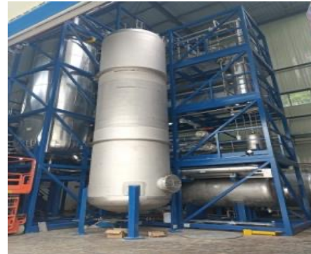
Distillation to remove radioactive impurities
