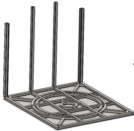
1 Install back column
