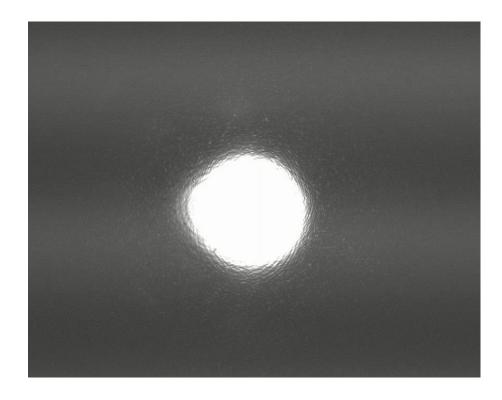
transmission of M2 when intra-cavity power at ~100 kW, TEM00 degenerated with high order mode
