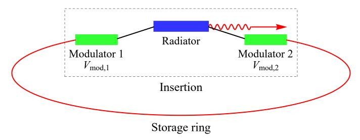
• Insertion: Two laser modulators, sandwiching the radiator, with modulation voltages  $V_{mod,1}$  and  $V_{mod,2}$ , to compress the microbunch length to 3 nm at the radiator. Bunching factor = 0.4.
